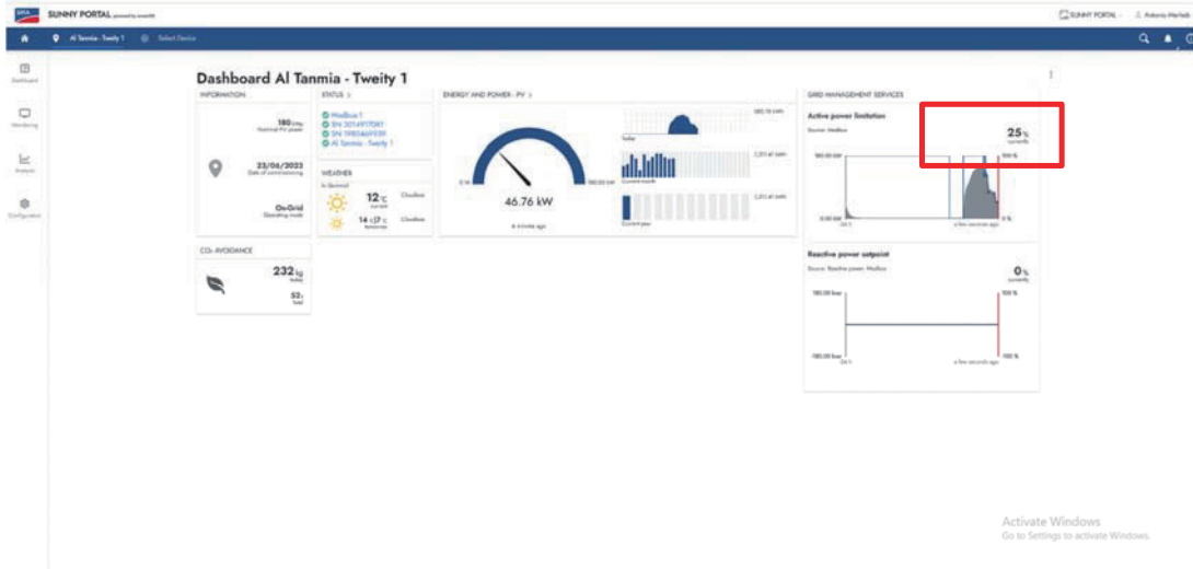
Fig. 12: SMA Monitoring platform showing 25% setpoint received from EMS
